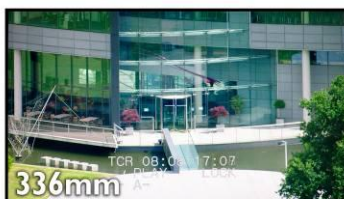
A typical 21x 7.8mm ENG lens using a x2 extender (21x7.8x2 = 336mm)
